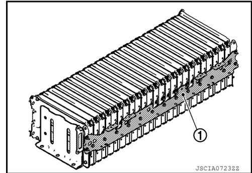
5. Fasten the rear module stack ① with a lashing belt ②.
