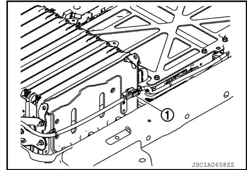
8. Install the Li-ion battery heater RR1 and RR2. Refer to [EVB-215, "LI-ION BATTERY HEATER : Disassembly and Assembly"](#).
