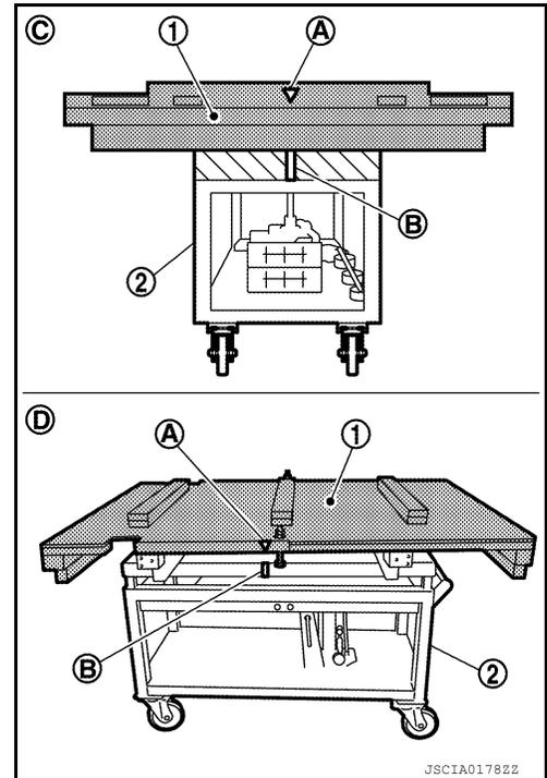
8. Set the pallet ① onto the Li-ion battery.
