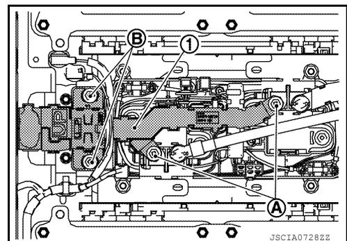
11. Remove the harness clips, then remove the battery member pipe (1).
