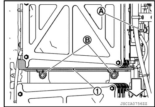
6. Remove mounting nuts (B) and then remove Li-ion battery heater RH2 (1).
