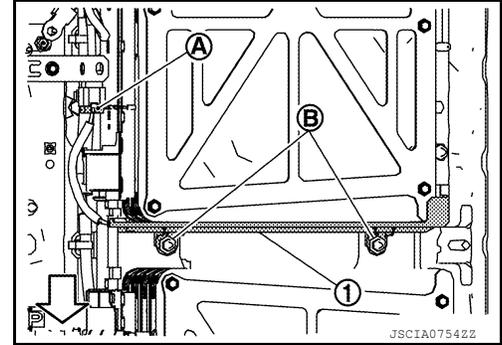
6. Remove mounting nuts ② and then remove Li-ion battery heater LH2 ①.
