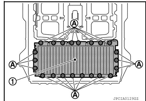
9. Follow the procedure below and remove the rear module stack from the battery pack.
