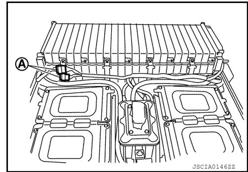
2. Measure voltages between positive terminal (A) of rear module stack and battery pack ground, and between positive terminal (B) of rear module stack and battery pack ground.
