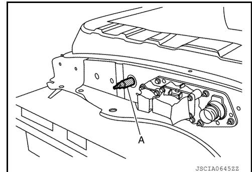
2. Install the gauge (A) of the air leak tester [SST: KV99111400 ( — )].
