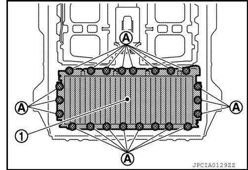
4. Tighten the mounting nuts (A), and then install the high-voltage harness (1), (2) onto the rear module stack.
