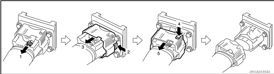
3. Disconnect the Li-ion battery heater harness connector (A).
