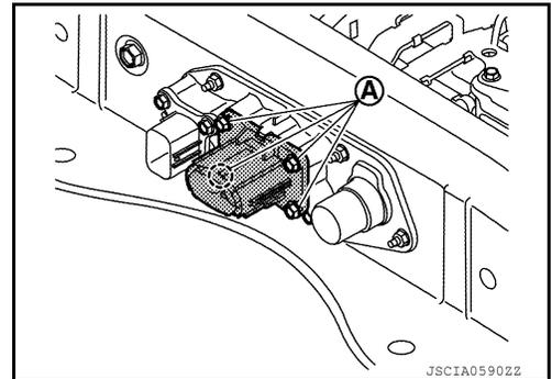
6. Disconnect the PTC heater harness connector (A).
