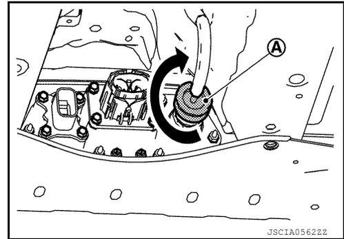
10. Install the Li-ion battery heater harness connector ①.
