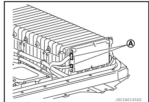
3. Remove the Li-ion battery controller mounting nuts (A), then remove the mounting bolts (B).
