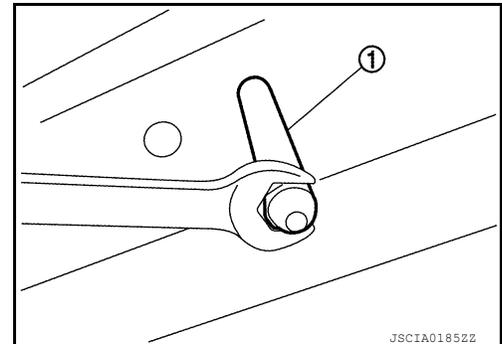
6. Install the Li-ion battery mounting bolts (A).
