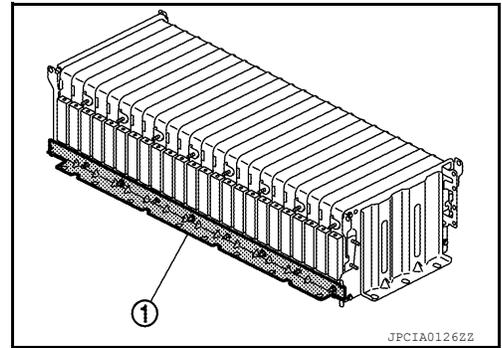
5. Remove the module terminal cover [SST: KV99111500 ( — )] (A).
