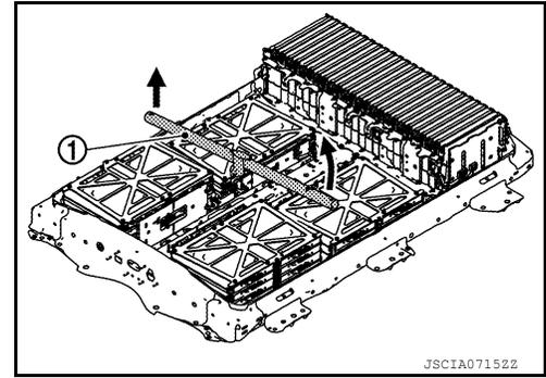
5. Disconnect Li-ion battery heater LH2 harness connector ①.
