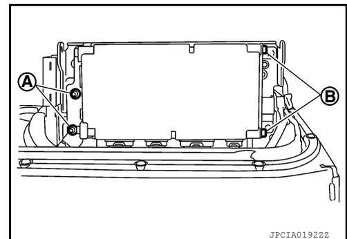
4. Disconnect the high-voltage harness connector (A), then remove the Li-ion battery controller.
