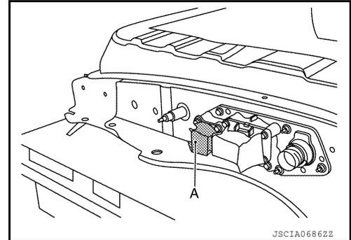
5. Use vinyl tape or similar means (A) to prevent air leakage from the breather.
