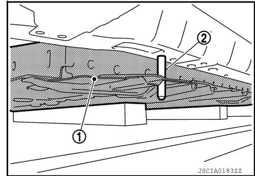
4. Tighten the Li-ion battery mounting bolts (4 bolts) (A), then remove the pallet.
