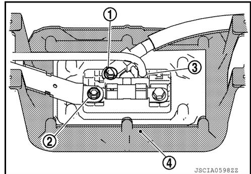
19. Remove the mounting nuts (A), then remove high-voltage harness (1) and (2).
