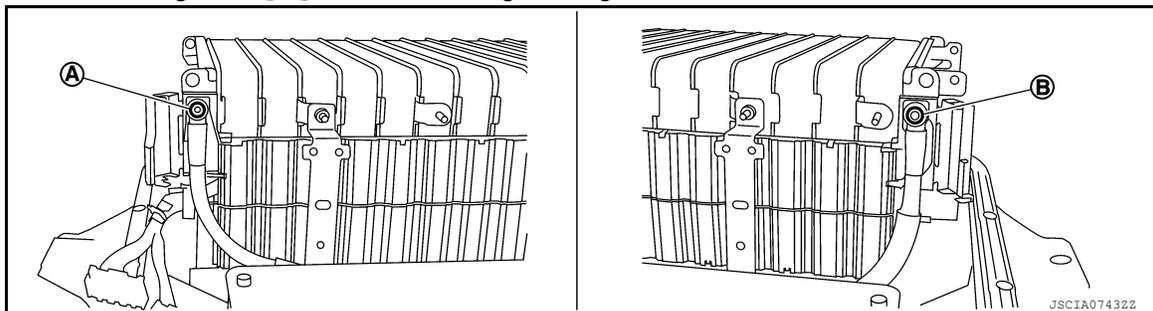
2. Measure voltages between positive terminal (A) of rear module stack and battery pack ground, and between positive terminal (B) of rear module stack and battery pack ground.
