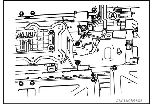
17. Remove the service plug switch bracket (1) mounting bolts (A).
