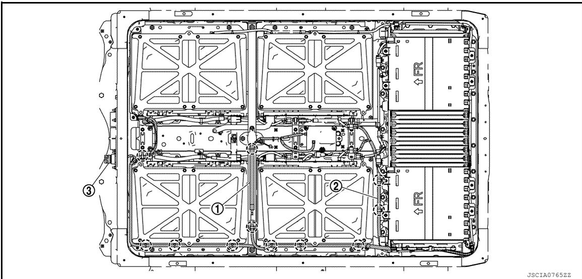
① Vehicle communications harness      ② Voltage detection harness      ③ Snap ring
