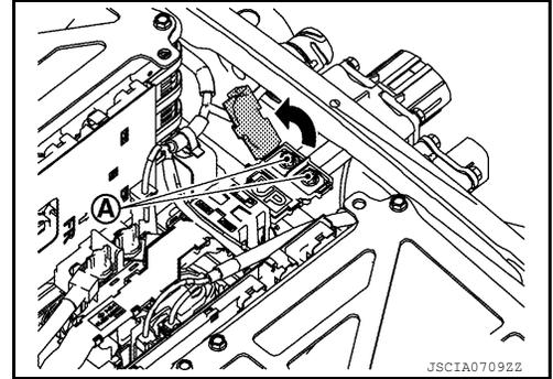
5. Remove the mounting bolt (A) and disconnect the high-voltage harness connector from the connector flange.
