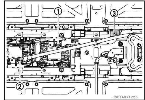
13. Remove the mounting nuts (A), and remove the bus bar ① and high-voltage harness ②.
