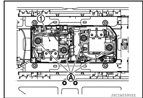
15. Disconnect the current sensor harness connector ①.
