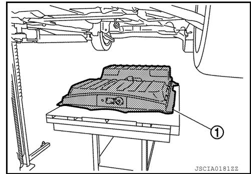
11. Lower the Li-ion battery from the lift table together with the pallet.
