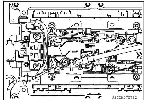
10. Remove the bus bar mounting nuts (A) and (B), and remove the bus bar (integrated with noise filter) (1).
