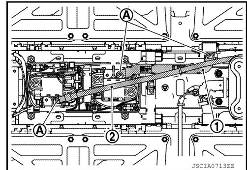
14. Remove the mounting nuts (A) and remove the junction box ①.
