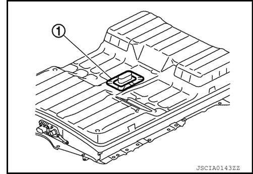
3. Remove the battery pack upper case mounting bolts ① and ground bolts ②.
