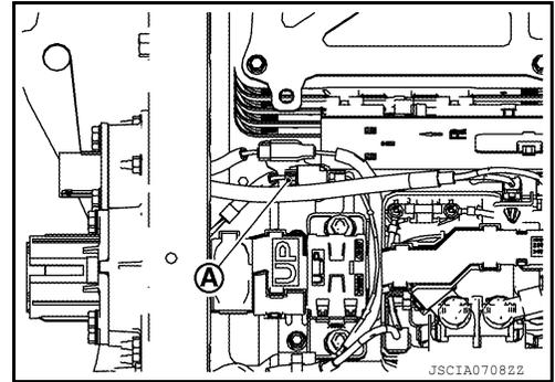
4. Open the bus bar cover and remove the high-voltage harness connector terminal mounting bolt (A).
