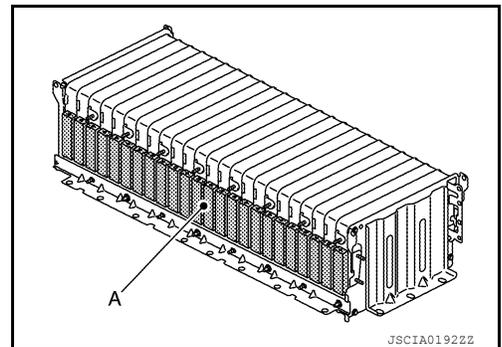
6. Follow the procedure below and install the bus bar module onto the rear module stack.
