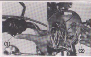
Fig. 5-33 (1) Horn button (2) Light green lead
