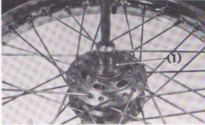
Fig. 4-5 (1) Bearing retainer wrench
