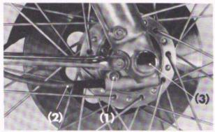
Fig. 4-2 (1) Setting screw (2) Speedometer cable (3) Front wheel axle
