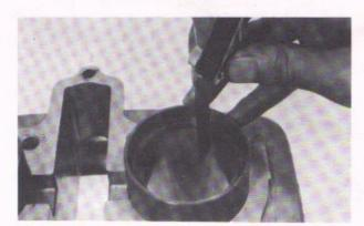
Fig. 3-13 Measuring piston ring end gap
