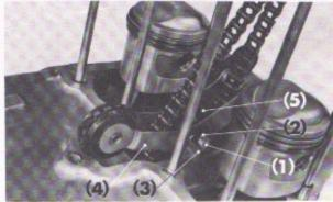
Fig. 3-55 (1) Bolt (2) Snap ring (3) Guide roller pin (4) Chain tensioner roller
