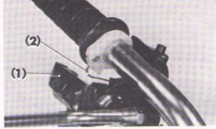
Fig. 4-49 (1) Switch (2) Throttle cable
