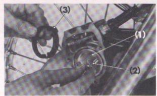
Fig. 4-15 (1) Pad A (2) 6mm bolt (3) Thrust plate guide
