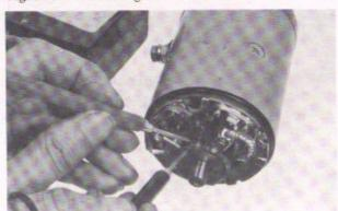
Checking armature coil Fig. 5-25
