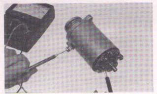
Fig. 5-24 Checking stator coil
