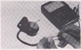
Fig. 5-29 Checking main switch for continuity
