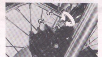
Fig. 2-17 (1) Front brake cable adjusting bolt
