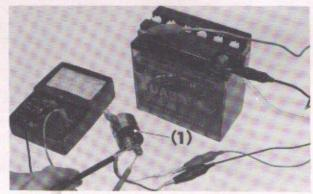
Fig. 5-28 (1) Starting magnetic switch
