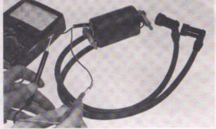
Checking ignition coil for continuity Fig. 5-3
