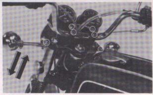
Fig. 2-36 (1) Checking front suspension
